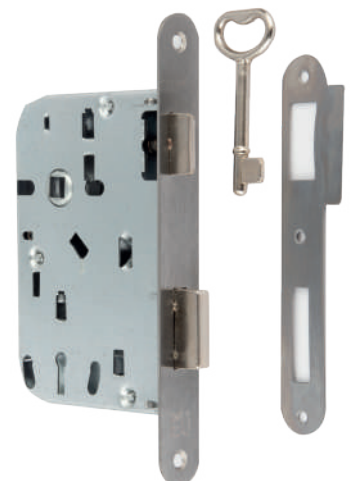
Key square edge lock at 68 between axles and 60 entrance. Material: Stainless Steel
